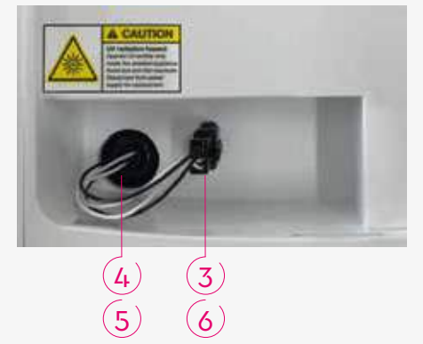
Fig. 12: UV lamp recess under the AQA drink Pro 20 cover
