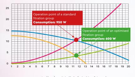
Load loss of an optimised hydraulic circuit in an 8×4 m pool Load loss of a stndard hyraulic circuit in an 8 × 4 pool EUROSTAR 100 pump performance curve EUROSTAR 50 pump performance curve
