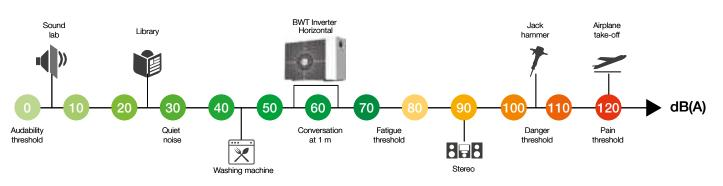
The scale above compare the acoustic power level of BWT Inverter horizontal with every events.
